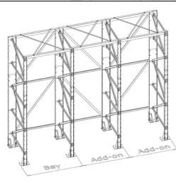
Approx total length is calculated by adding the starter bay to the sum of the add-on widths.
